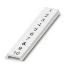
Zack Marker strip, flat, Strip, white, labeled, Printed vertically: consecutive numbers 1 ... 10, 11 ... 20, etc. up to 91 ... 100, mounting type: snapped, for terminal block width: 3.5 mm, lettering field size: 5.15 x 3.5 mm, Number of individual labels: 10
